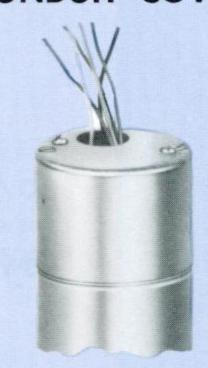
Conforms to the National Electric Code standards. It is provided with a  $\frac{7}{8}$  inch hole for a half inch connector. For one element overspeed and underspeed switches this cover is placed over the screw terminals. For two element switches, six leads are brought out of the cover. No conduit cover is available for three element switches.
