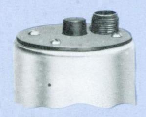
Sometimes military specifications, contaminated atmosphere, or high voltage condition requires the speed switch to be fitted with a MS Connector. One element overspeed and underspeed switches are furnished with MS 3102R-10SL-3P, three (3) pin connector. Two element switches are furnished with MS 3102R-14S-6P, six (6) pin connector. Three element switches are furnished with MS 3102R-18-1P, ten (10) pin connector which is wired 3DDB as shown below. Other wiring arrangements must be specified.
