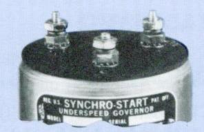
For most applications screw terminals are the most practical method of wiring the speed switch to the device that it controls. Three terminals (normally open, normally closed and common) are furnished with one element overspeed and underspeed switches. Two element switches are furnished with six screw terminals (normally open, normally closed and common for each element).
