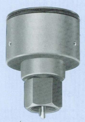
GO STYLE. Direct mounts on SAE tachometer accessory drive found on most engines manufactured in the USA. Four different DRIVE SHAFTS are avaiable: .187 in. diam., .152 in. diam., .203 in. diam., and .104 in. square. The flexible drive shaft compensates for misalignment.
